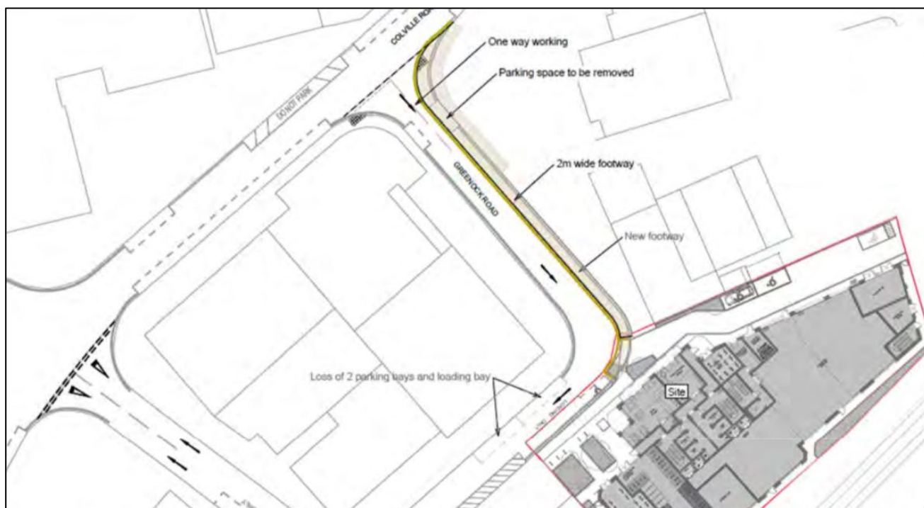
Figure 34: Indicative Upgrades to Greenock Road
